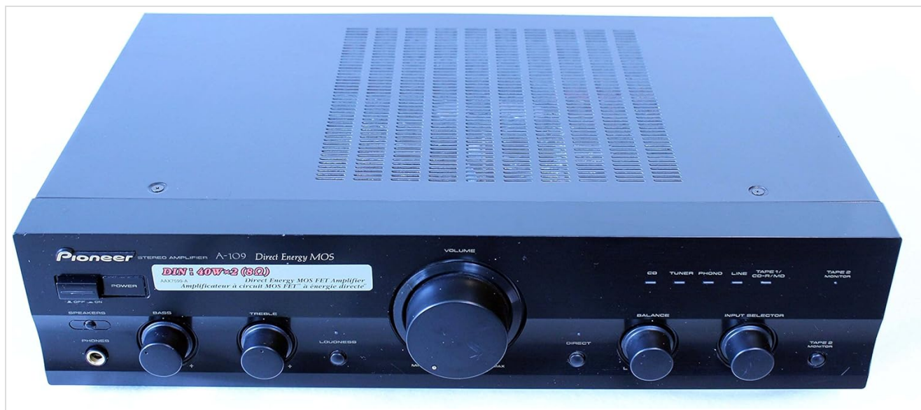
Figure 4.1: Front view of the Pioneer A-109 Hifi Amplifier. This image displays the power button, input selectors (CD, Tuner, Phono, Line, Tape 1, Tape 2), volume knob, bass and treble controls, loudness button, balance knob, and headphone jack.
