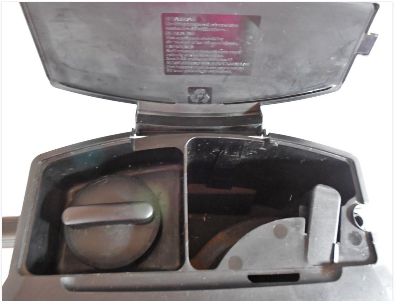
Figure 4: Top view of the machine, illustrating the separate water reservoirs for drip coffee and espresso. The espresso reservoir is on the left.
