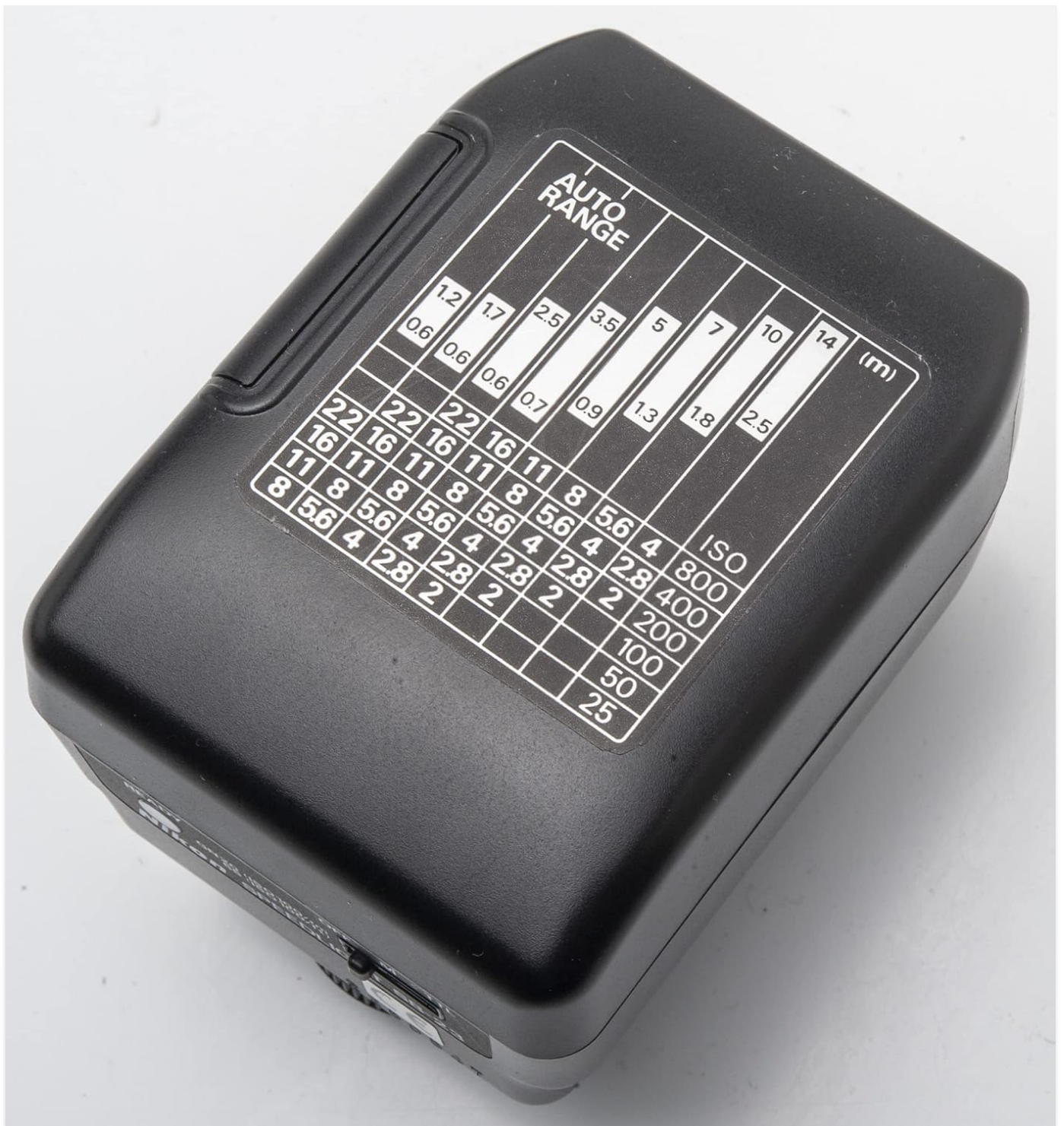
Figure 5: Close-up view of the Auto Range table located on the side of the Nikon SB-23 Speedlight. This table provides aperture values (f-stops) for different ISO settings and flash-to-subject distances in meters and feet.
