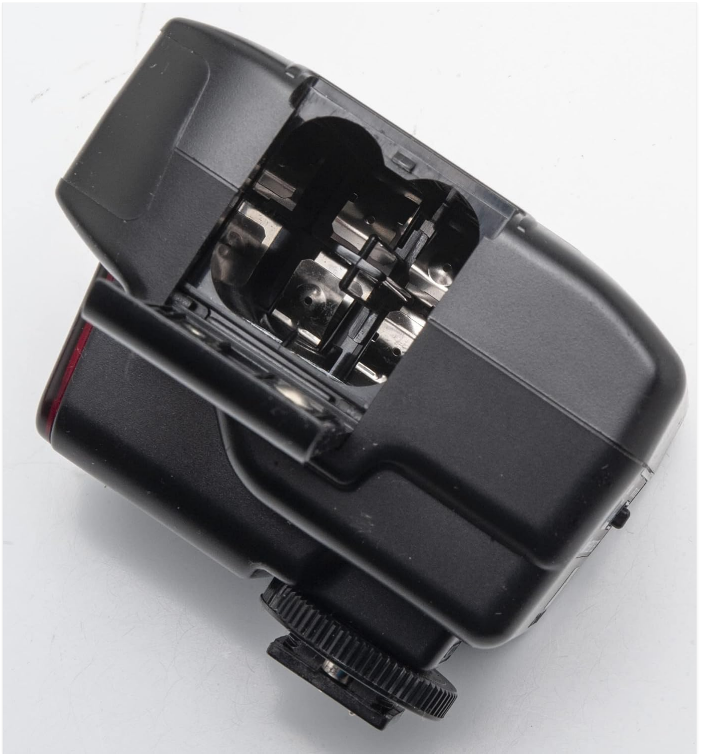
Figure 4: View of the Nikon SB-23 Speedlight with the battery compartment open, showing the slots for four AA batteries and polarity markings.
