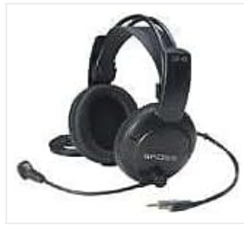
Figure 2: The Koss SB40 headset showing its dual 3.5mm audio and microphone plugs for connection to a computer.
