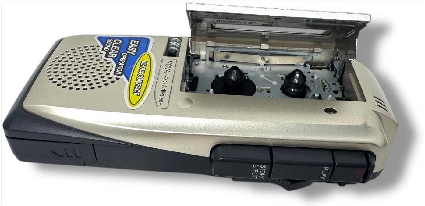
Figure 1: Top view of the Olympus J300 Microcassette Recorder with the cassette compartment open, showing the tape reels and recording mechanism. The device features a speaker grille on the left and control labels like "EASY CLEAR SOUND" and "ULTRA-COMPACT" on its surface.
