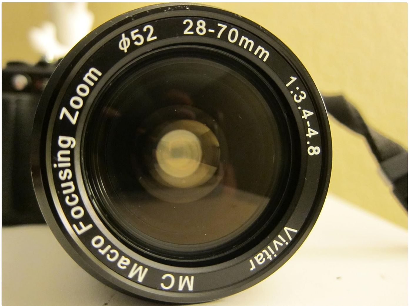
Figure 7: Front view of the Vivitar 28-70mm lens, displaying the focal length range (28-70mm), aperture range (1:3.4-4.8), and filter thread size ( \phi 52 ).
