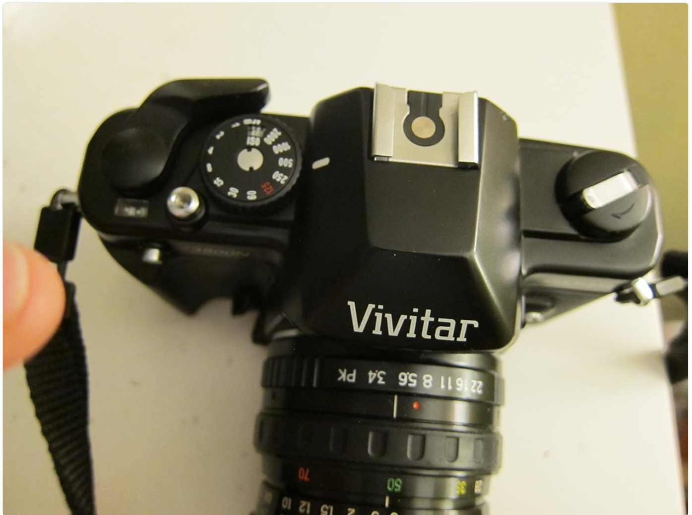
Figure 6: Top view of the Vivitar V3800N camera, clearly showing the shutter speed dial with various settings, the hot shoe for external flash, and the film advance lever.
