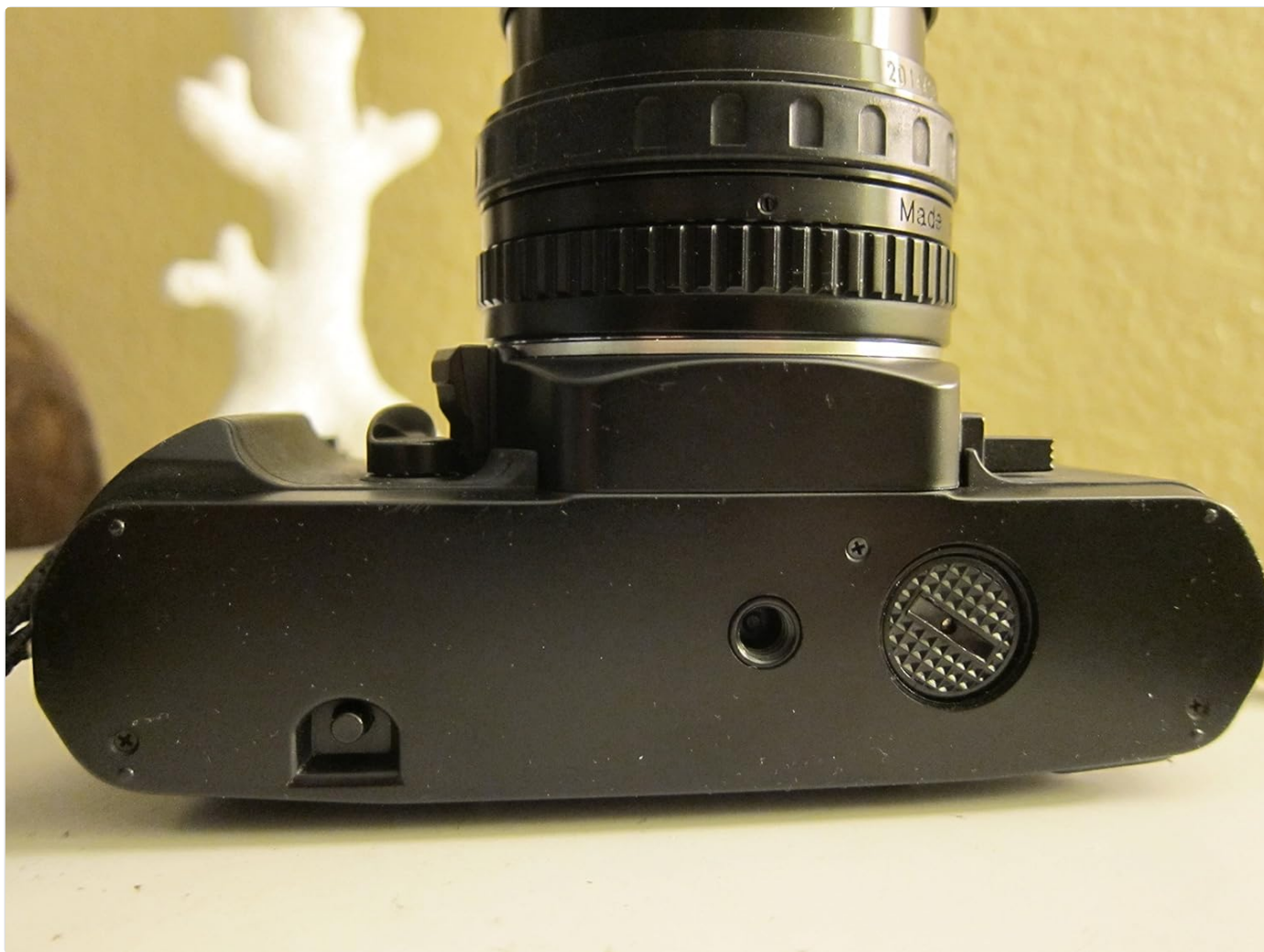
Figure 2: The bottom of the Vivitar V3800N camera, highlighting the circular battery compartment cover on the right and the tripod mount in the center.
