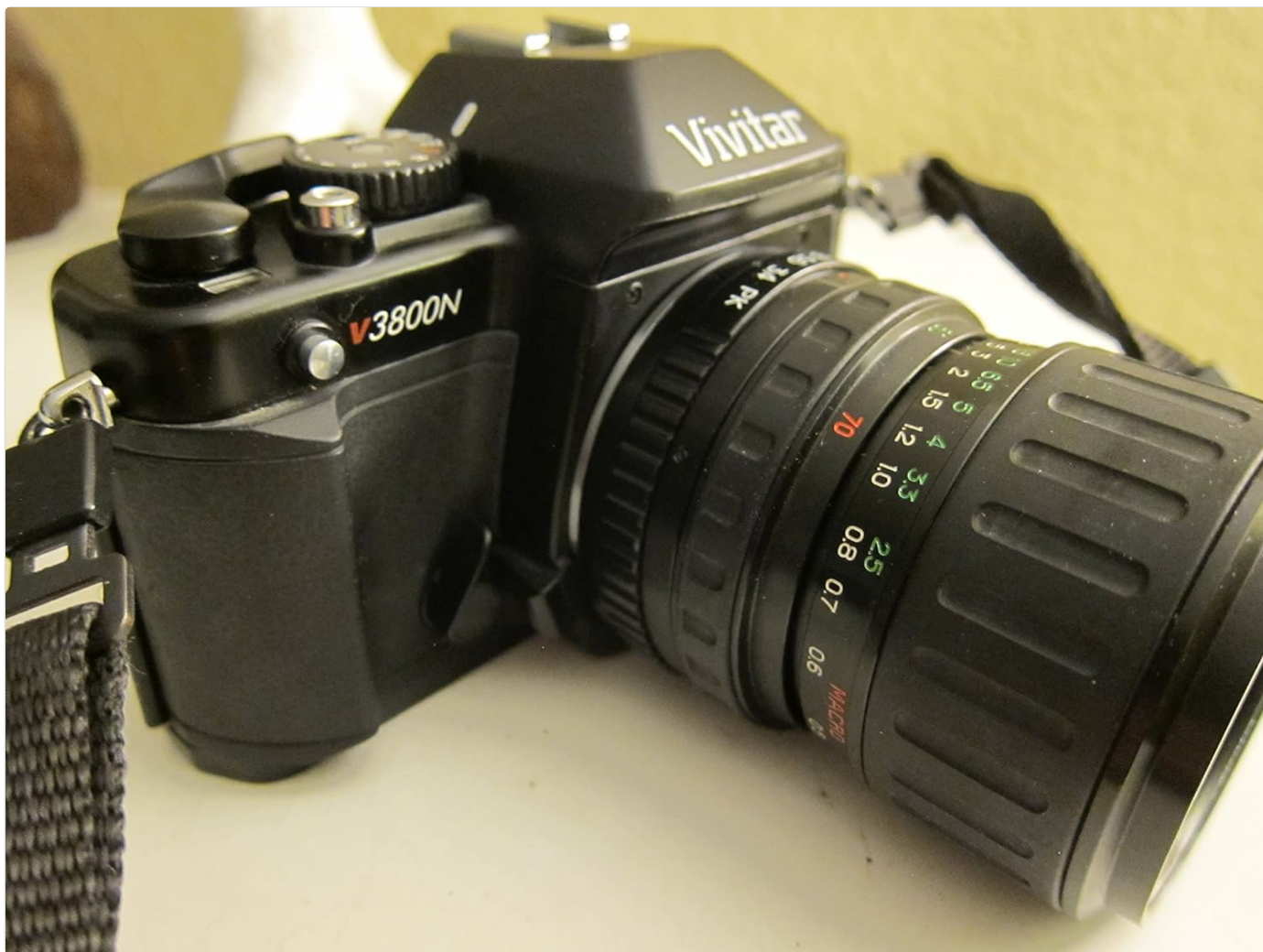
Figure 5: Side view of the Vivitar V3800N camera, illustrating the attached 28-70mm lens with its focus and zoom rings clearly visible. The camera's V3800N model designation is also visible.
