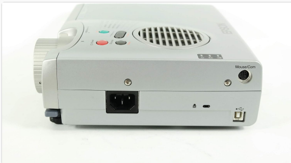
Figure 3: Right Side View. This view shows the AC power input socket and the Mouse/Com port, which is used for connecting to a computer for control and mouse functionality.
