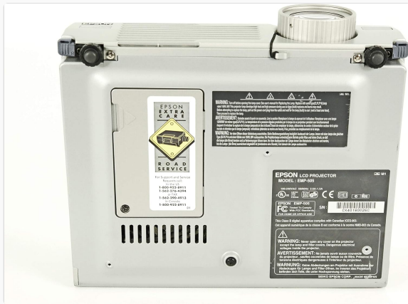
Figure 5: Bottom View. The underside of the projector displays regulatory labels, serial number information, and mounting points for ceiling or wall arm installations.
