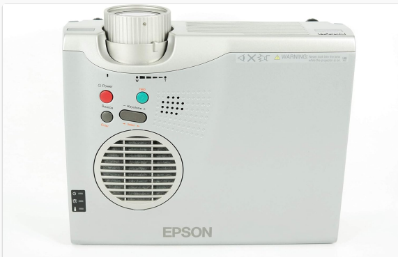
Figure 4: Top Control Panel. The top panel includes essential control buttons such as Power, Source selection, Keystone adjustment, and navigation buttons for menu interaction.
