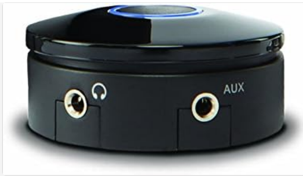
Figure 3: The control pod, featuring the master volume dial, power indicator, headphone jack, and auxiliary input.
