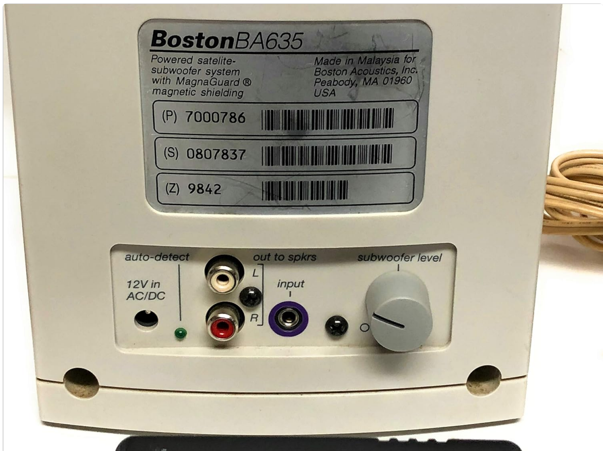
Image 2: Rear panel of the BA635 subwoofer, showing the "12V in AC/DC" power input, "out to spkrs" outputs for satellite speakers, and "input" for audio source.
