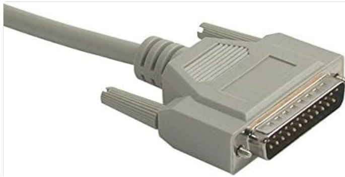
Image: A close-up view of the DB25 Male connector, showing the 25 pins.
