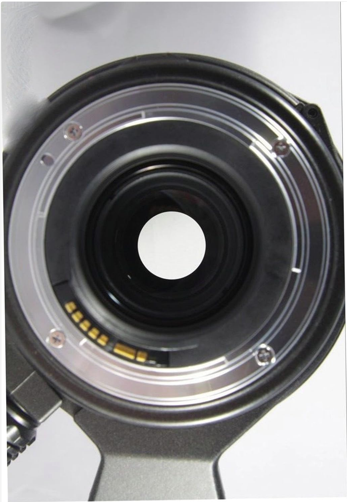
Image: Rear view of the Tamron AF200-400mm lens, showing the Canon-AF mount with electronic contacts. This is where the lens connects to the camera body.
