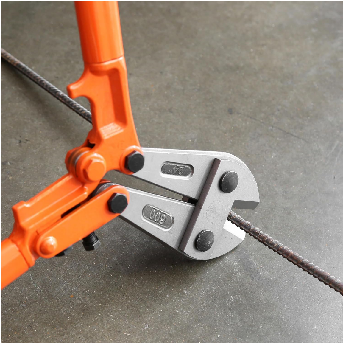
Image 4.1: The bolt cutter jaws positioned to cut a metal rod, demonstrating proper placement for maximum leverage.
