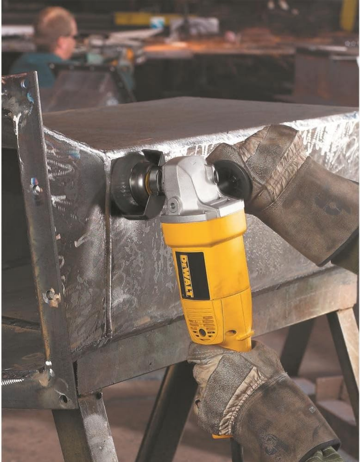
Figure 2: The DEWALT DW831 Angle Grinder being used for material removal, demonstrating proper grip with the side handle.
