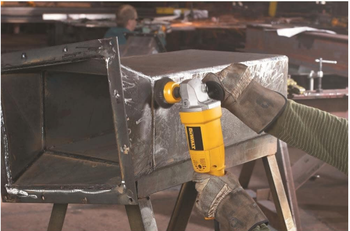
Figure 3: The DEWALT DW831 Angle Grinder being used to clean a metal surface, illustrating the tool's application in metal preparation.
