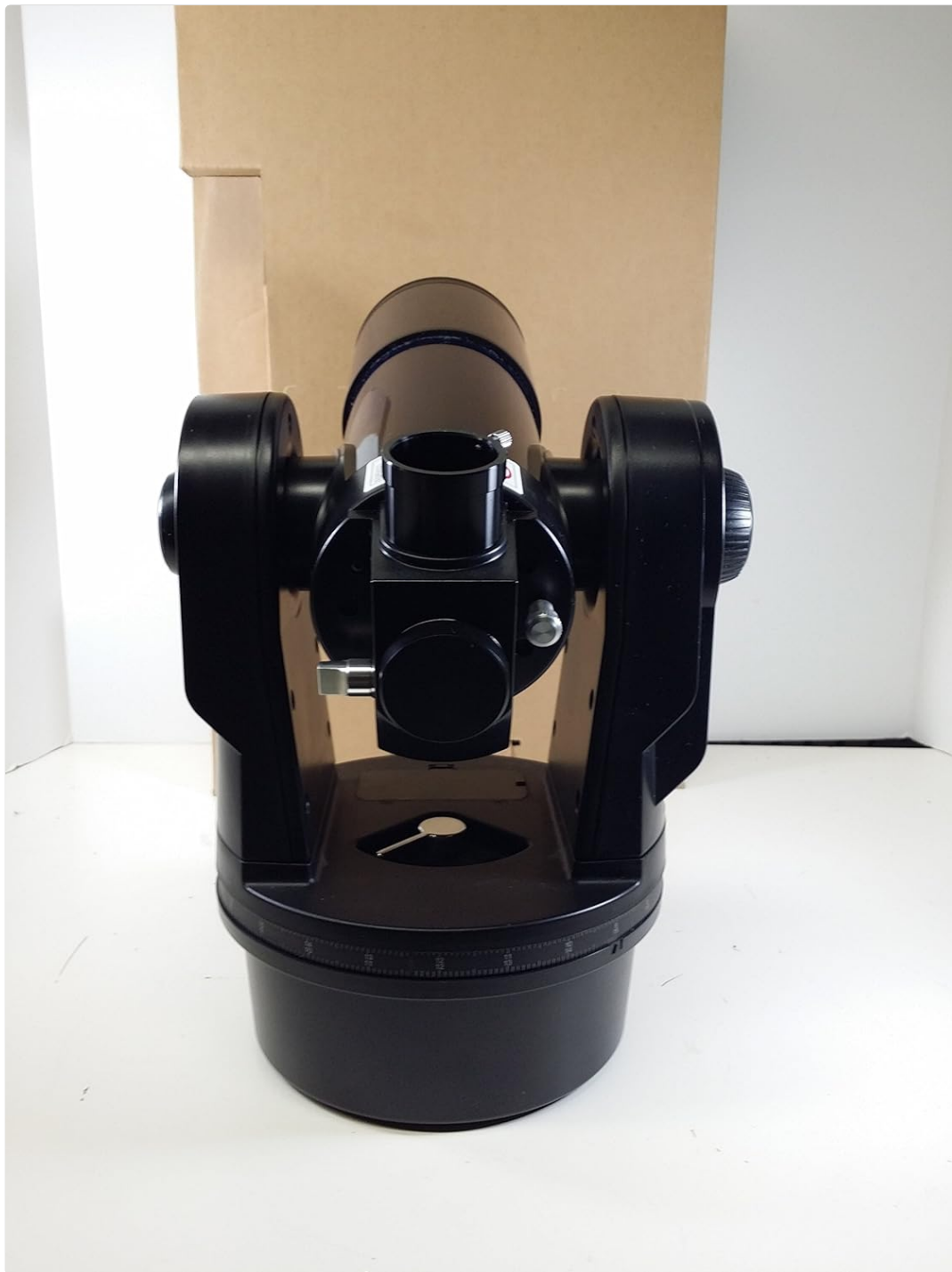
Figure 5.1: Close-up of the Meade ETX60AT Telescope showing the focus knob and flip-mirror lever.
