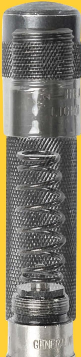
Figure 3: An illustration showing the internal spring mechanism of the center punch, which allows for adjustment of tension to produce lighter or heavier marks on various surfaces.
