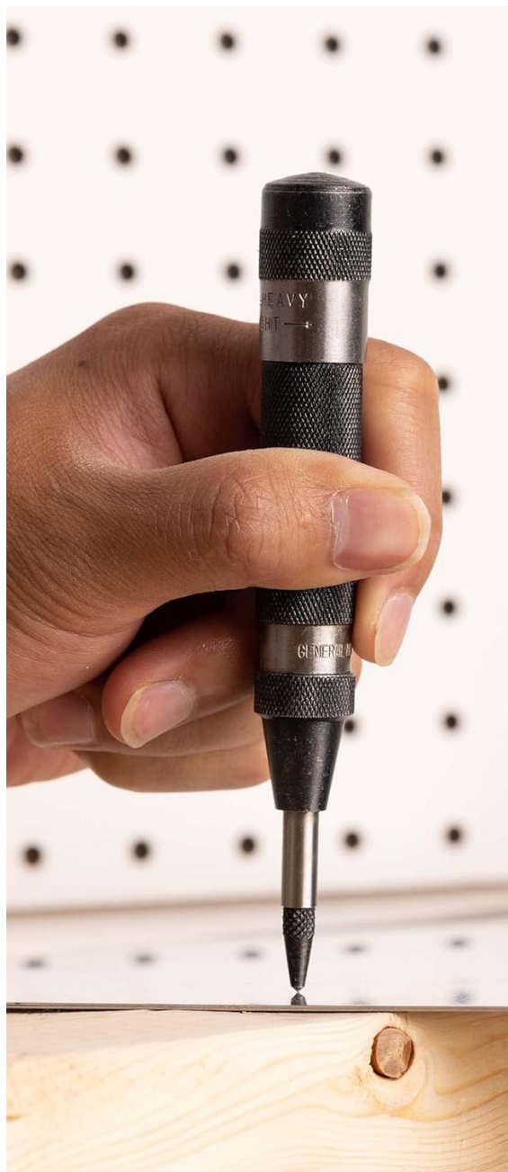
Figure 5: An image demonstrating the automatic center punch being used to mark a point on a wooden surface, highlighting its application for various trades.
