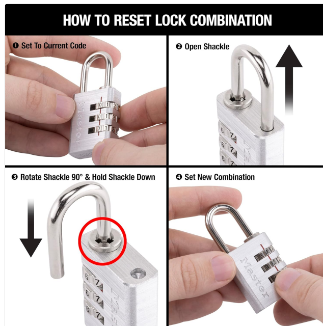
Image: A four-panel diagram illustrating the steps to reset the lock combination, showing the lock being opened, shackle rotated, pressed down, and new combination set.
