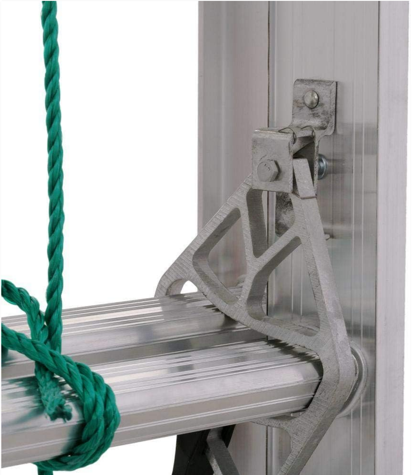
Figure 3: Close-up view of the heavy-duty spring-loaded lock mechanism on the Werner D1220-2 extension ladder. These locks ensure the fly section is securely held in place when extended.
