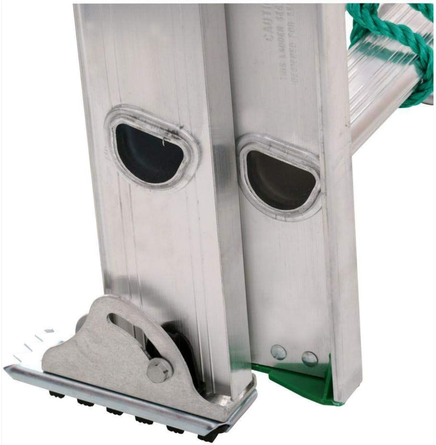
Figure 5: The Shu-Lok feature on the ladder's feet, allowing them to be positioned flat for hard surfaces or in a spur position for soft ground, enhancing stability.
