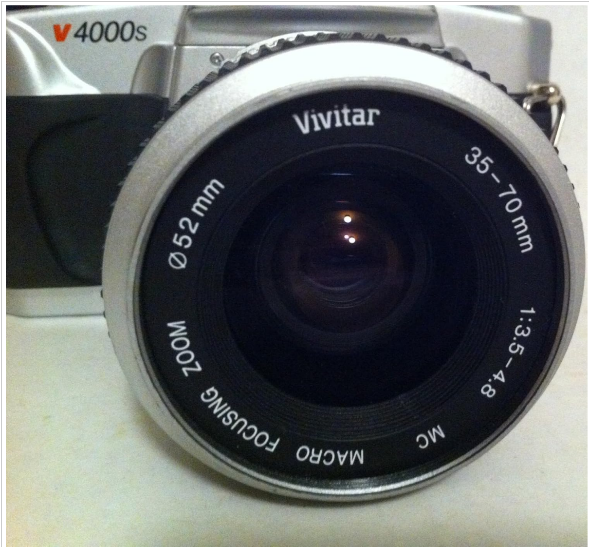
Figure 2: Front view of the 35-70mm lens, showing focusing and aperture controls.
