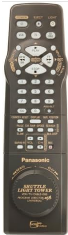
Image 4.3: Universal illuminated remote control for the Panasonic PV-V4640 VCR. The remote features various buttons for power, channel selection, volume, playback controls, menu navigation, and a distinctive jog/shuttle dial at the bottom.
