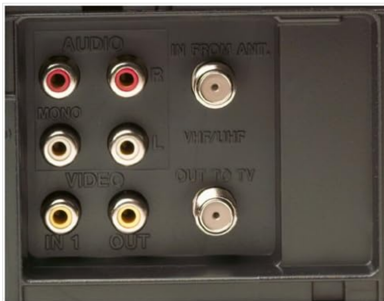
Image 4.2: Rear view of the Panasonic PV-V4640 VCR. This image highlights the various audio and video input/output ports, including RCA jacks for audio (L/R) and video (IN/OUT), and coaxial connectors for antenna/cable input and TV output.
