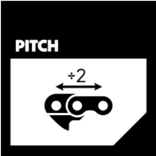
Image: Chain Pitch. Illustrates the distance between three consecutive rivets divided by two.
