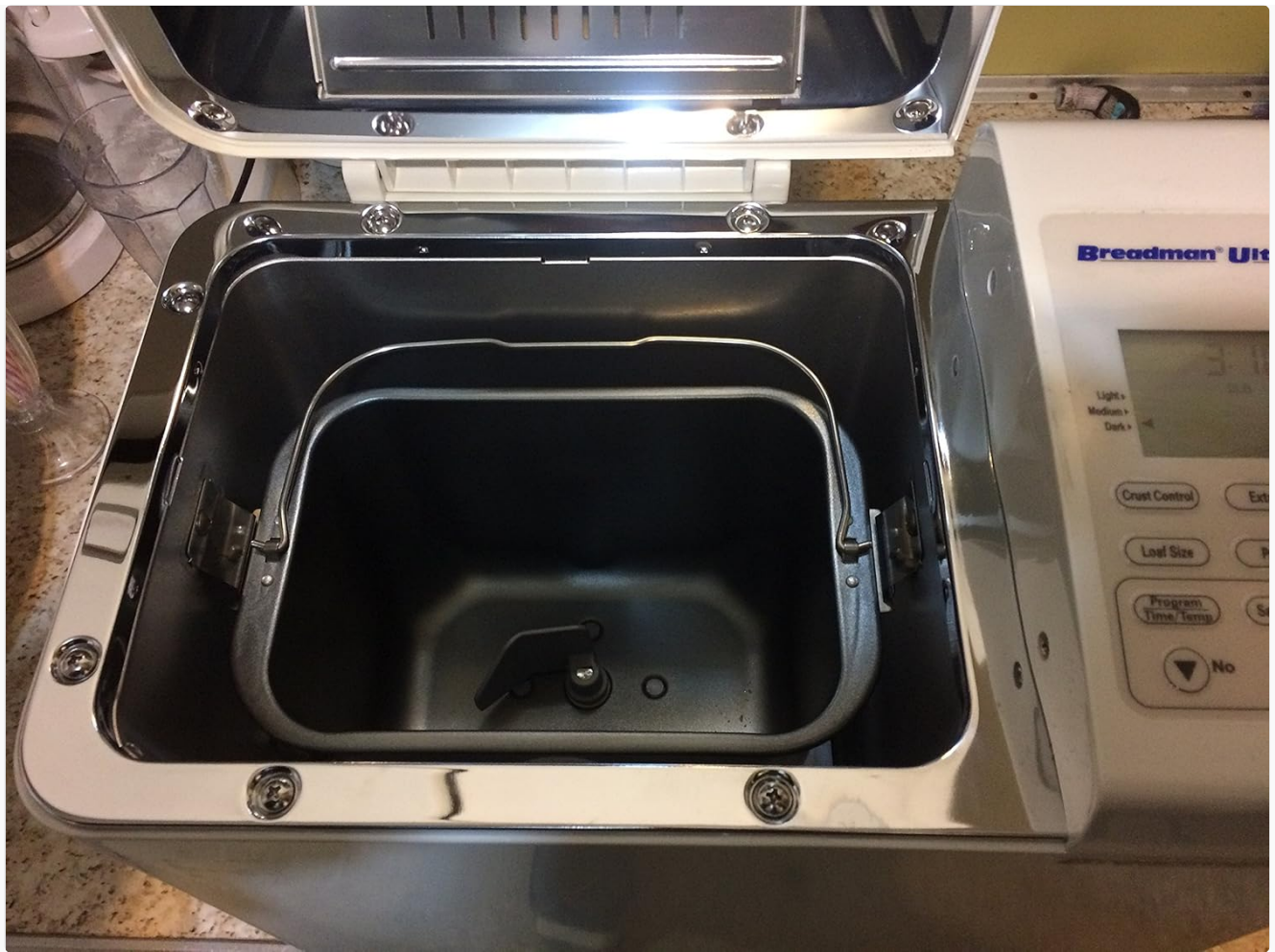
Figure 3: The interior of the bread machine with the nonstick bread pan securely in place. The kneading paddle is visible at the bottom of the pan.
