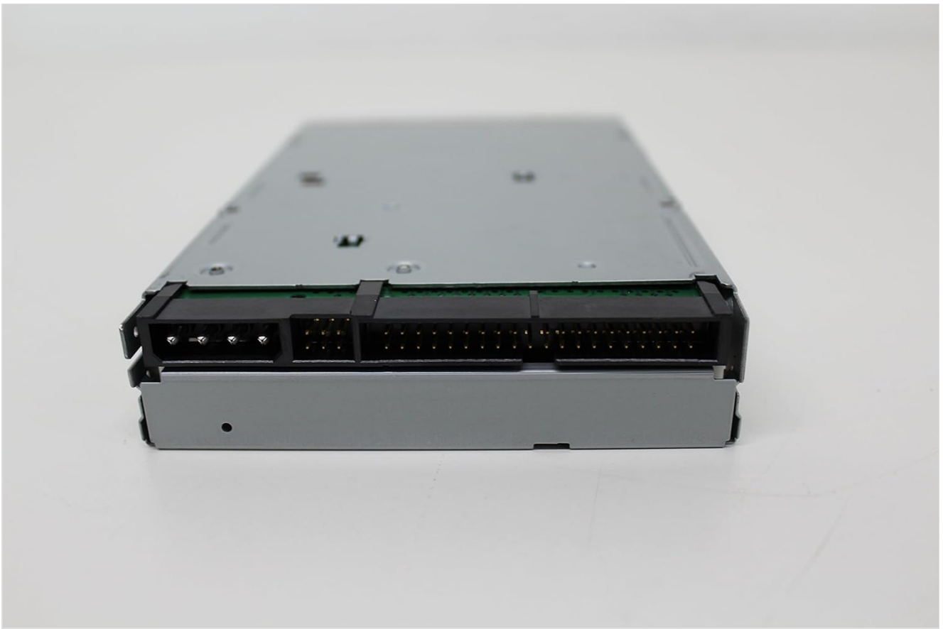
Figure 3: Rear view of the drive, illustrating the ATAPI data connector and the 4-pin power connector.
