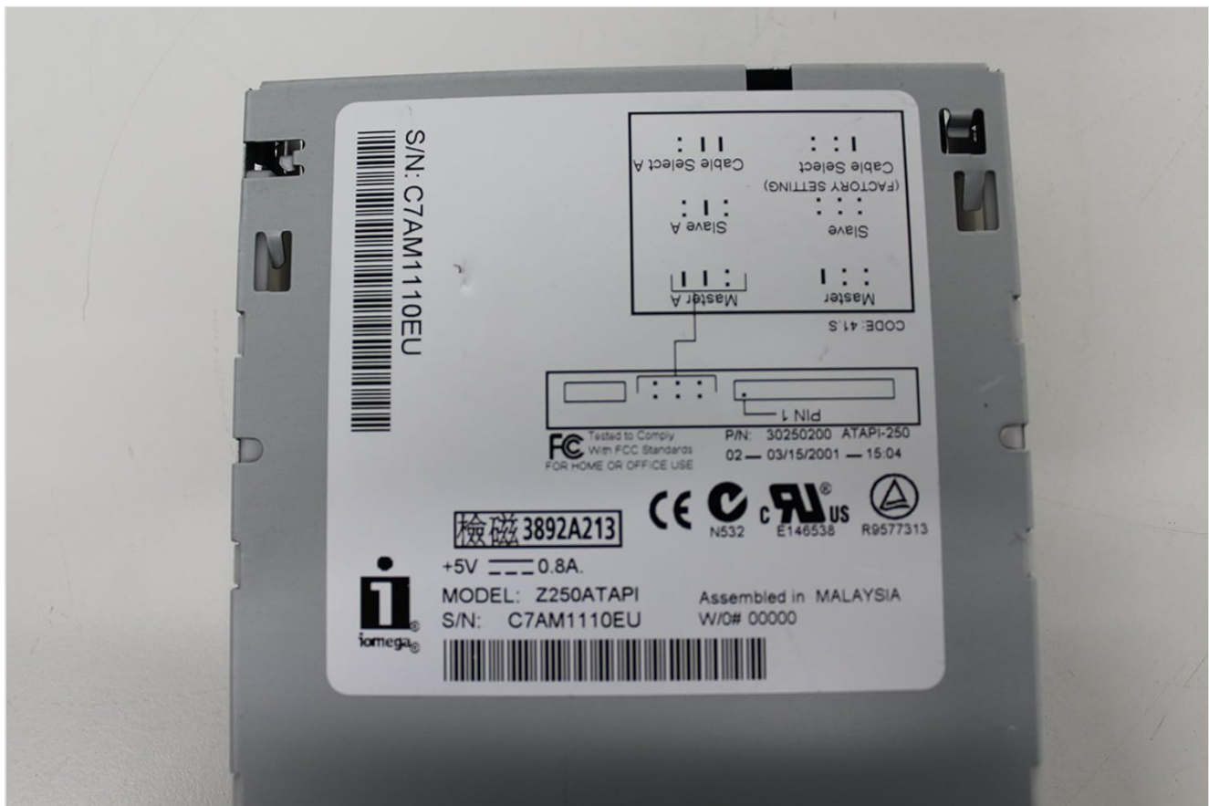
Figure 2: Drive label showing jumper settings for Master, Slave, and Cable Select. The model number is Z250ATAPI and serial number is C7AM1110EU.
