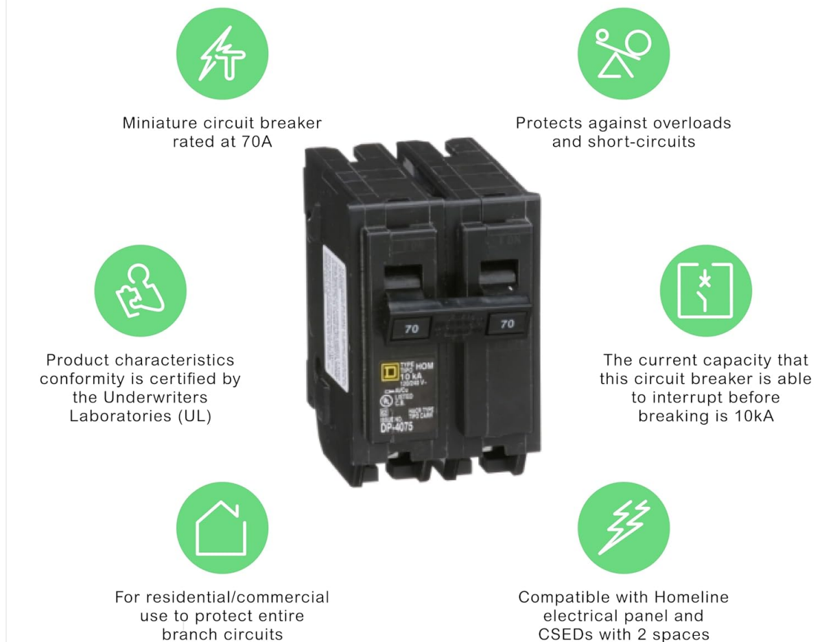
Figure 2: Technical benefits of the Square D Homeline 70 Amp 2-Pole Mini Circuit Breaker, highlighting its miniature size, overload/short-circuit protection, UL certification, 10kA breaking capacity, residential/commercial use, and compatibility with Homeline panels.
