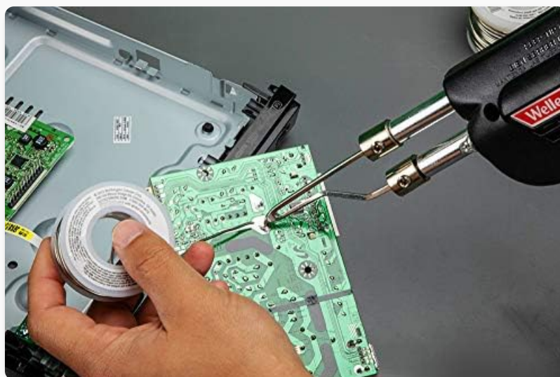
Figure 5: The soldering gun actively melting solder on a circuit board, demonstrating its effectiveness in practical applications.
