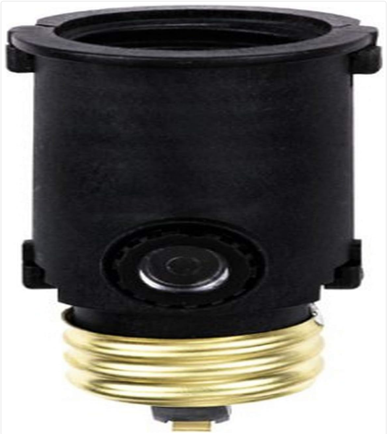
Image: The Intermatic NE1C Screw-In Photo Control, showing its screw-in base and integrated photocell sensor. This device is designed to be inserted into a standard light socket, with an incandescent bulb then screwed into the control itself.
