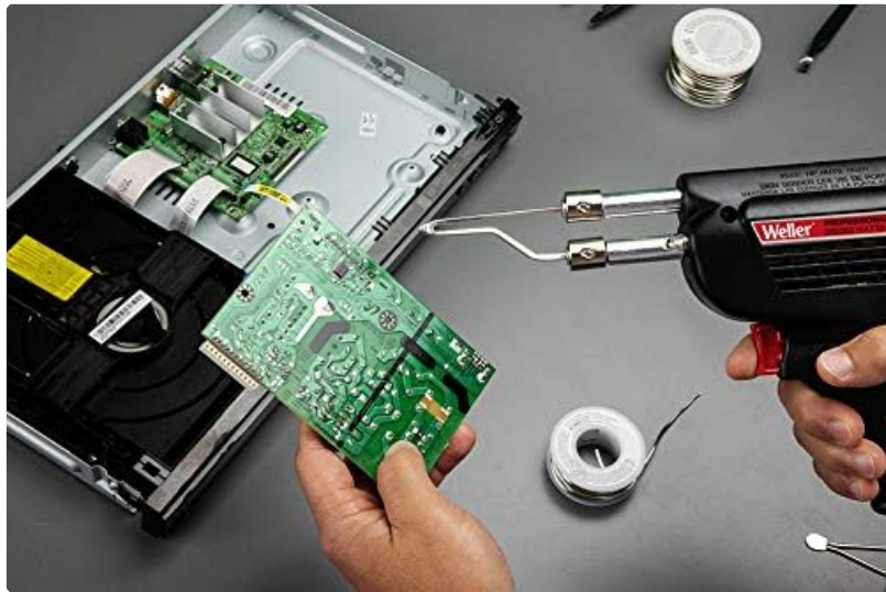
Figure 5: Soldering a circuit board using the Weller D550.
