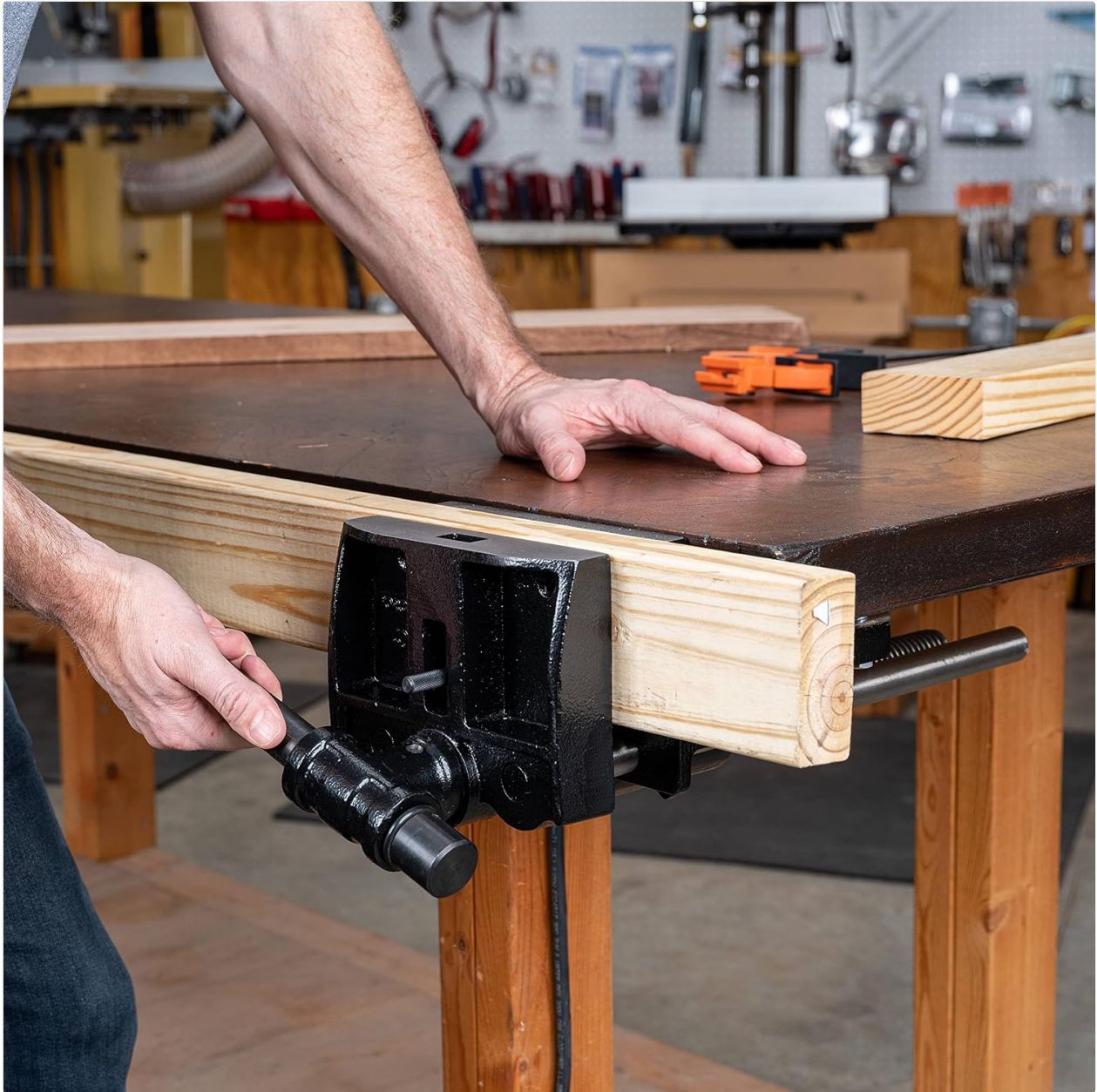
Figure 3: Demonstrating the vise holding a wooden workpiece.
