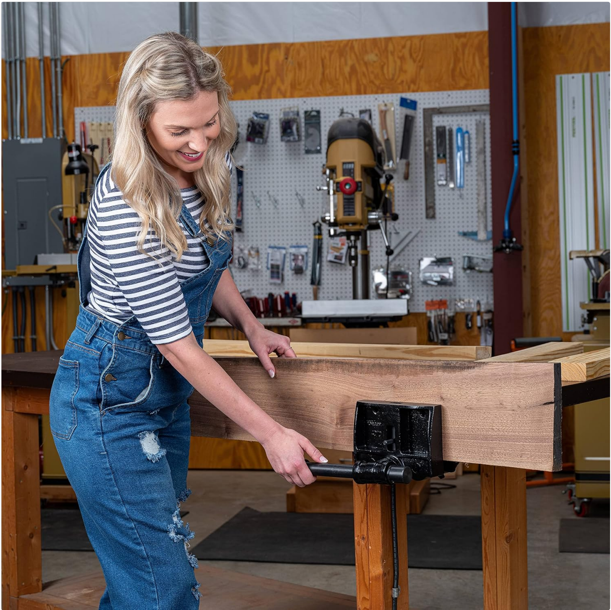
Figure 4: Using the vise to secure a larger wooden beam.
