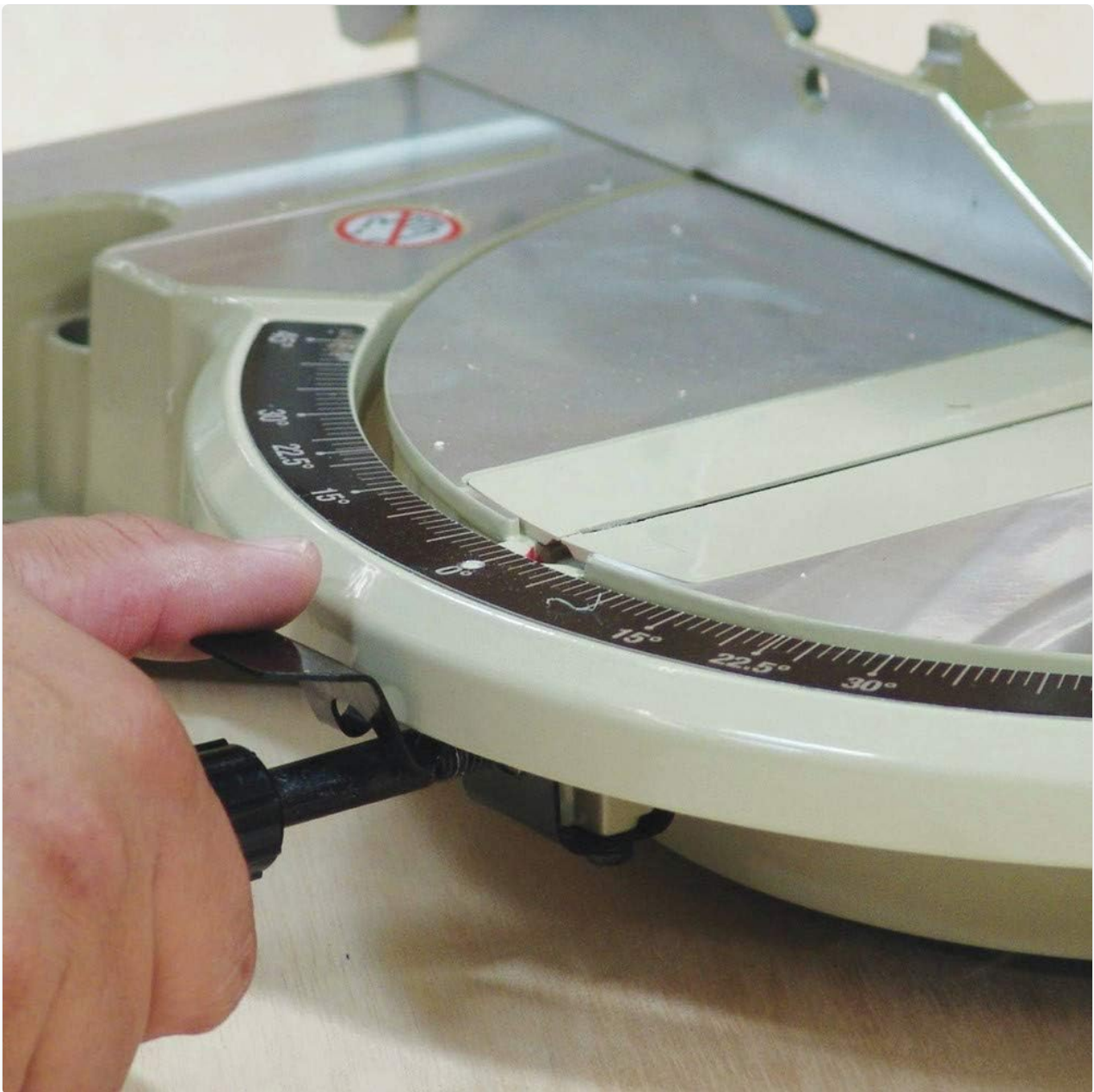
Figure 4: A hand demonstrating the adjustment of the miter angle lock, allowing the user to set the cutting angle.
