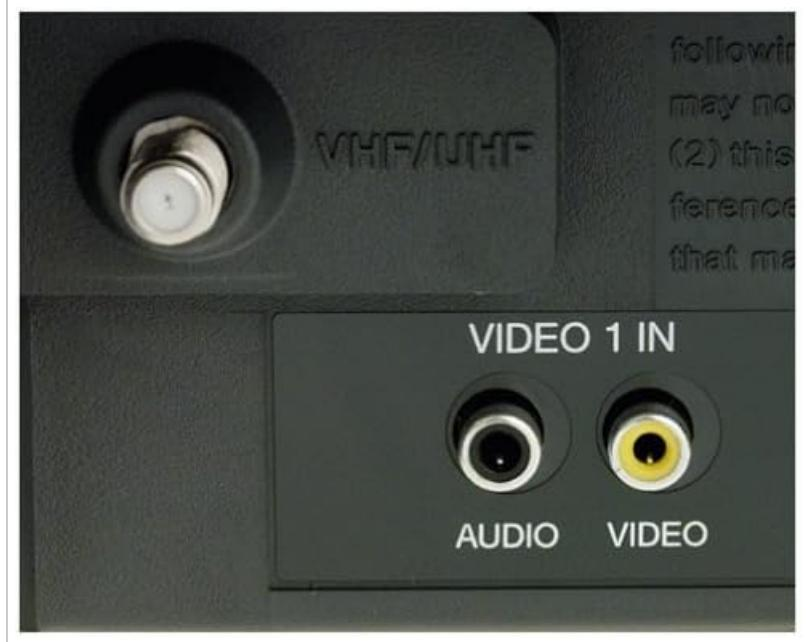
This image displays the rear connection panel of the television. It features a coaxial input for VHF/UHF antenna connection and a set of RCA jacks labeled 'VIDEO 1 IN' for composite video (yellow) and audio (white) input.
