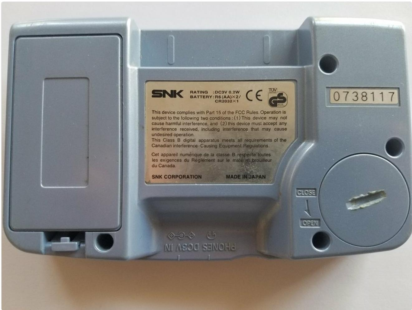
This image shows the rear of the SNK NEOGEO Pocket Color Console. The large rectangular cover for the battery compartment is prominent on the left. A product label with SNK branding, rating information (DC3V 0.2W, BATT: R6(AA)x2 / CR2032x1), and regulatory compliance text is affixed to the center. A serial number '0738117' is visible on the upper right. The 'OPEN' and 'CLOSE' indicators for the battery cover are also visible.
