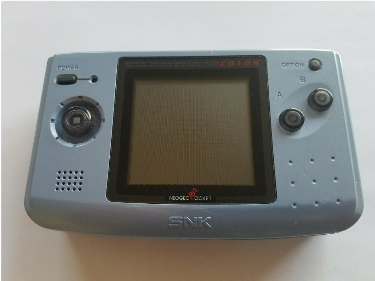
This image displays the front of the SNK NEOGEO Pocket Color Console. Visible components include the central LCD screen, the circular thumbstick on the left, the 'A' and 'B' action buttons on the right, and the 'POWER' and 'OPTION' buttons located at the top left and right corners respectively. The console's speaker grille is also visible on the lower left.
