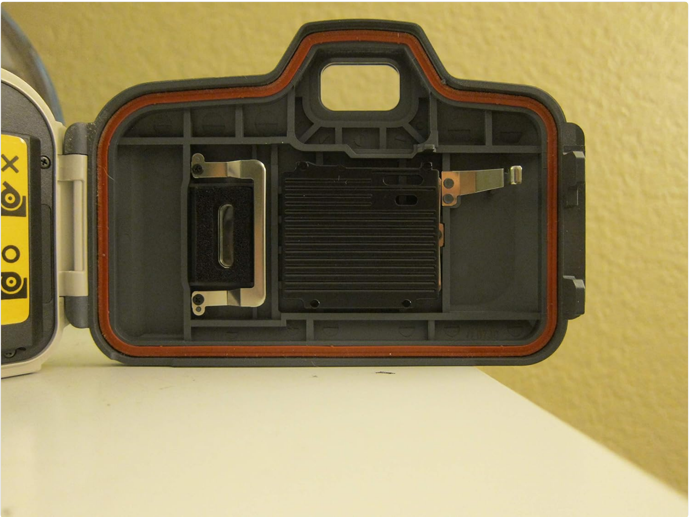
Figure 1: View of the open battery compartment, showing where to insert the CR123A battery.
