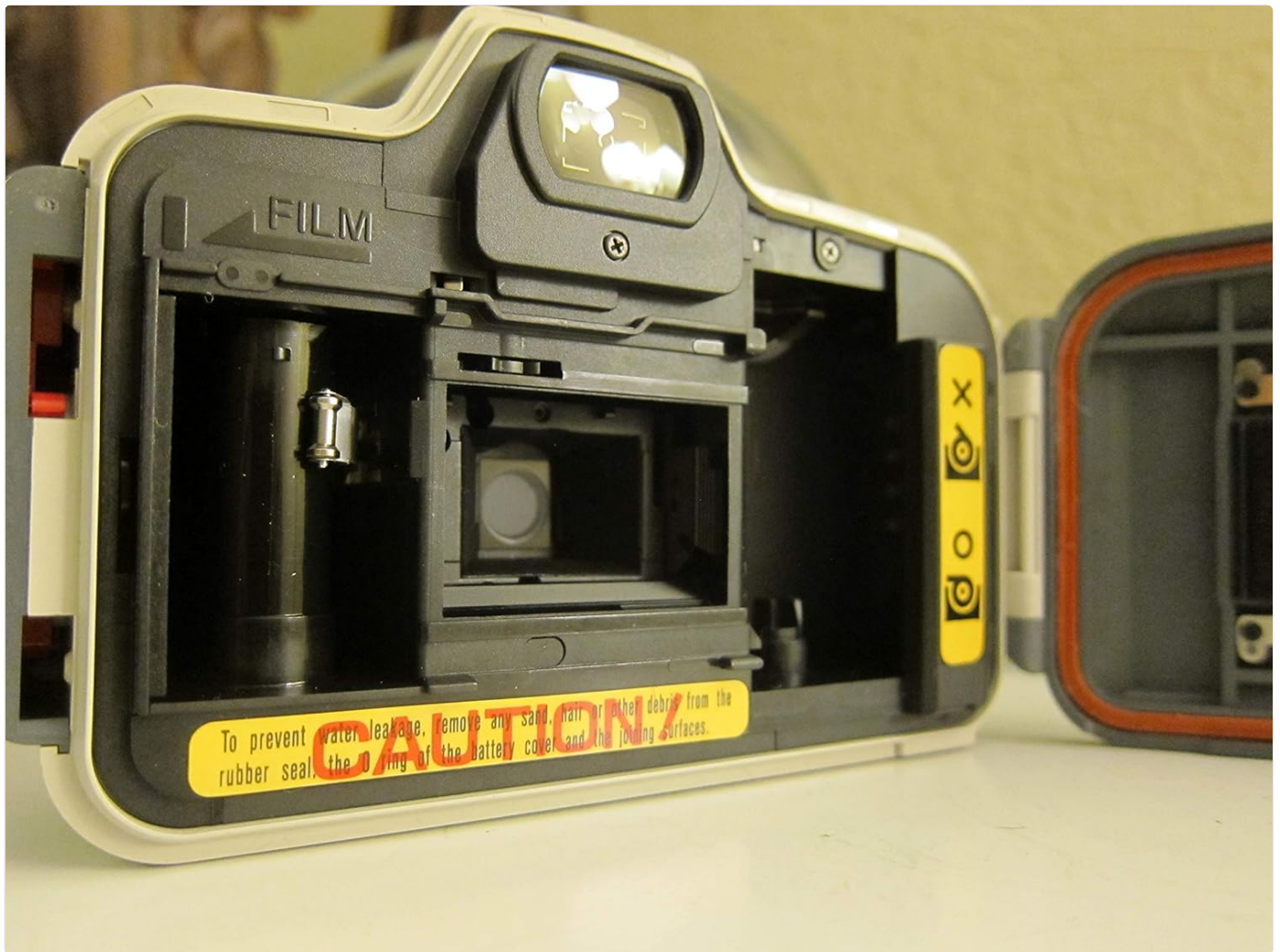
Figure 2: The camera's film compartment, showing the film chamber on the left and the take-up spool on the right.
