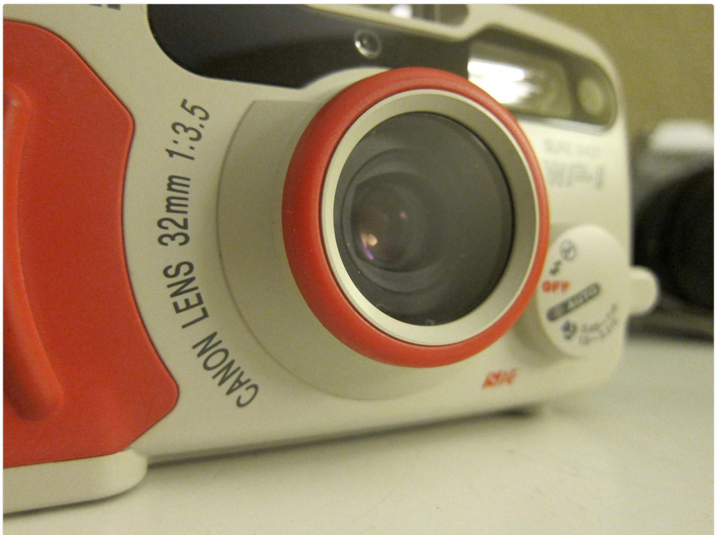
Figure 3: The lens and surrounding dial, used to power the camera on and off, and select shooting modes.
