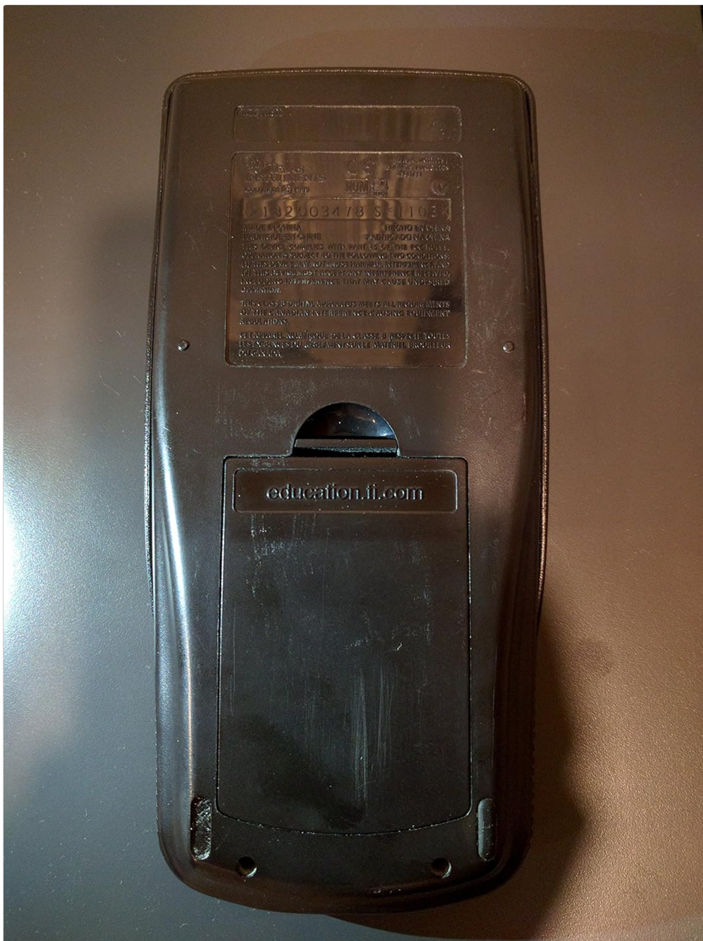
Figure 2.2.1: Rear view of the TI-86 Graphing Calculator, showing the battery compartment. This is where the four AAA batteries are inserted for power.
