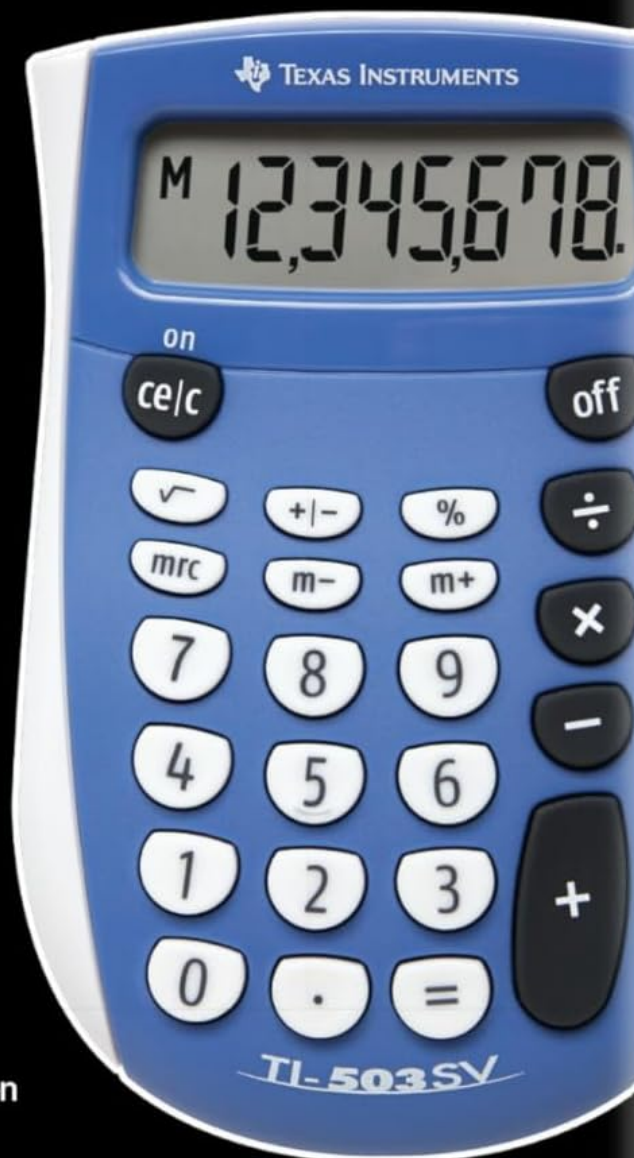
Figure 2: The TI-503 SV calculator as packaged, highlighting its SuperView™ display, battery power, and auto-shutoff features.
