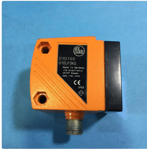
Figure 3: Side view displaying the model number (O1D100 O1DLF3KG), manufacturer (ifm electronic), and IP65 protection rating.
