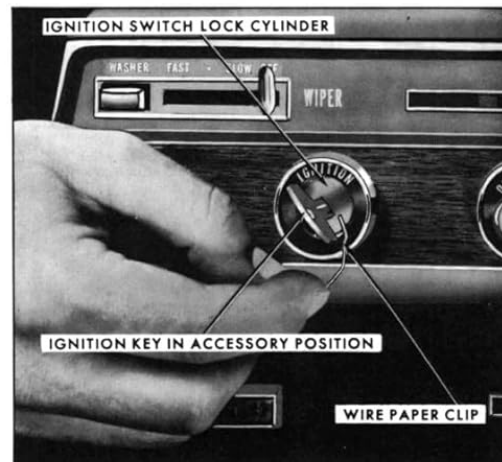
Fig. 10E-9. Ignition Switch Lock Cylinder Removal (61LM-7619)
