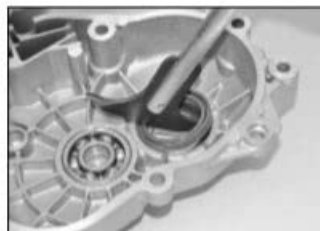
6.17c ... using a seal hook or screwdriver...
