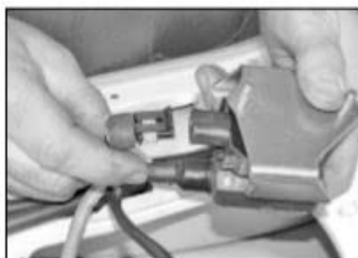
3.15b ... then draw the coil out and disconnect the wiring connector
