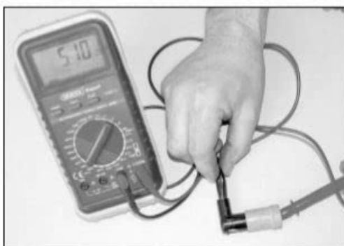
3.7 Measuring the resistance of the spark plug cap
