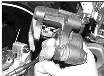
6.9 You should be able to push the piston in using finger pressure
