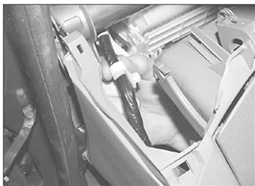
26.16b . . . then unclip the harness from the back of the facia . . .
