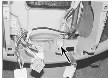
26.15b Remove the central screw (arrowed)
