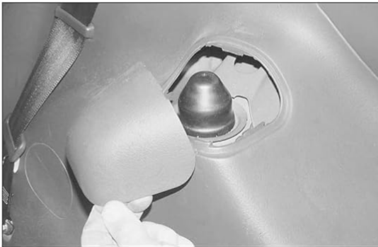
10.1a Prise off the plastic trim panel inside the boot . . .
