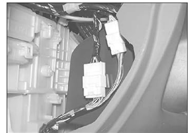
26.16a Disconnect the wiring plugs inside the glovebox aperture . . .
