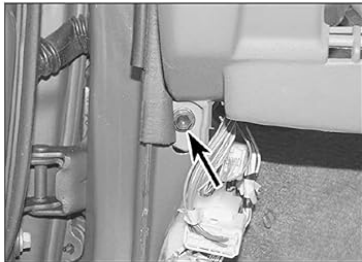
26.15a One of the lower section bottom mounting bolts
