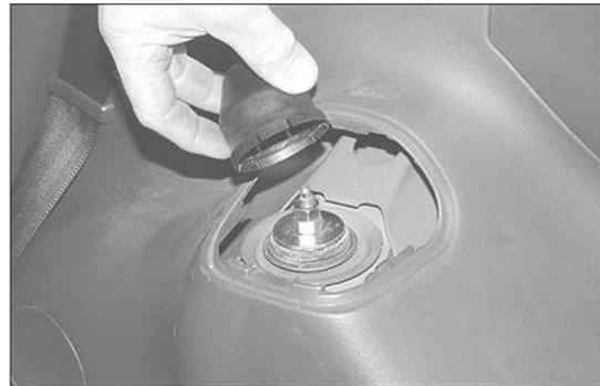
10.1b . . . then pull off the shock absorber rubber cover
