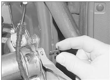
26.15c Prise out the plastic clip at each end . . .
