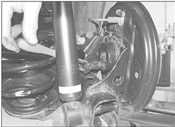
9.6 Disconnect the ABS sensor wiring plug using a screwdriver
