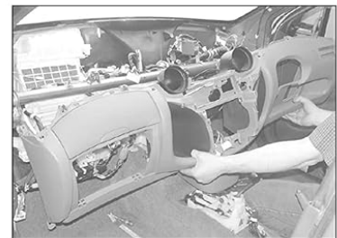
26.16d With everything detached from it, lift out the facia lower section
