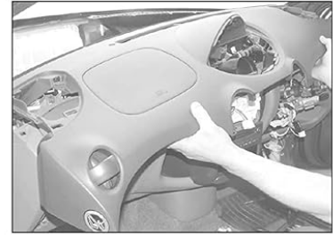
26.10 Push the facia upper section upwards to release the clips
