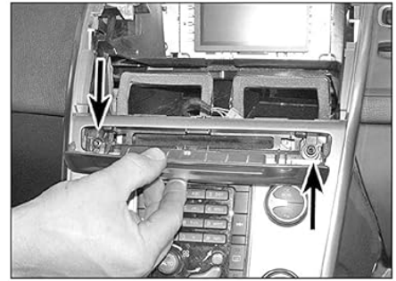
26.11 Remove the panel and then the screws (arrowed)
