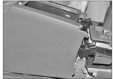
26.16 Remove the main section of the centre console
