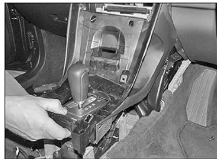
26.17b ...and lift off the support panel
