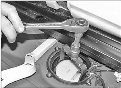
7.9a Remove the locking collar
