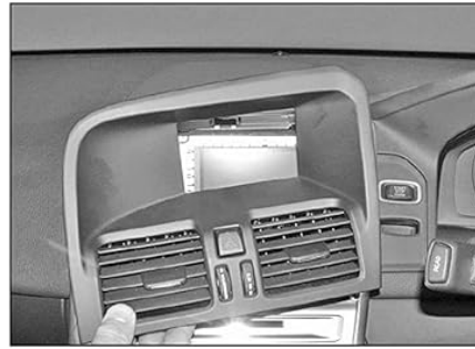
26.10b ...remove the air vent panel
