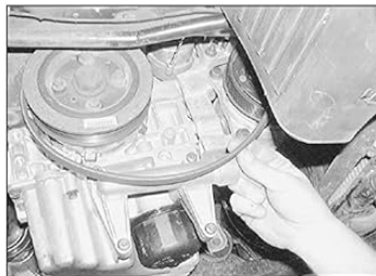
32.5 The drivebelt can now be slipped off all its pulleys
