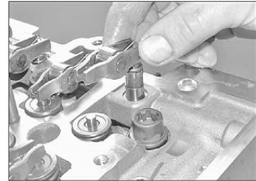
11.6b ... then refit the tappet to its original bore, and lay the follower over its respective valve
