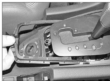
27.6b . . . and slide out the retaining frame
