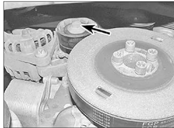
27.3a Turn the drivebelt tensioner clockwise using a spanner on the pulley centre bolt (arrowed) . . .
