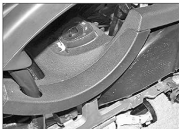
27.7 Prise up the panel beneath the handbrake lever
