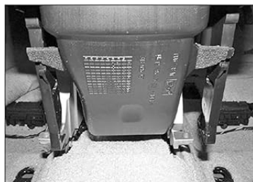
27.11a Lift the air duct from its mountings, and pull it rearwards
