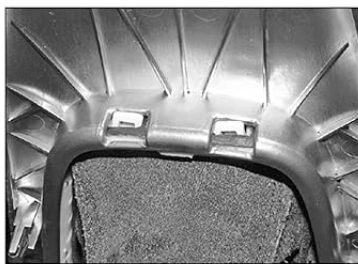
27.5 Unclip the gear lever gaiter/frame from the trim
