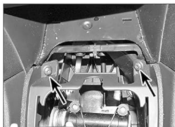
27.10a Undo the 2 Torx screws at the front of the console (arrowed) . . .
