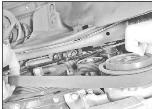
22.6 Place a wrench on the tensioner pulley center bolt and rotate it counterclockwise - 2.4L engine shown
