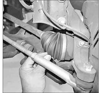
16.14 Inspect the inner and outer driveaxle boots for loose clamps, cracks or signs of leaking lubricant
