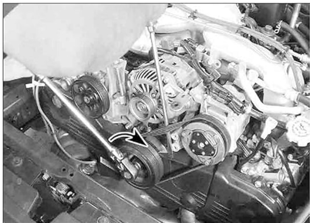
19.16 Typical "stretchy belt" removal technique
