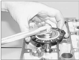
10.41c Angle-tightening the cylinder head bolts
