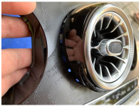
PUSH THE TOP UPWARDS INTO THE AIR VENT
