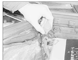
31.6a Pull out the automatic transmission fluid level dipstick ...
