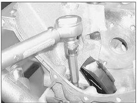
10.42 Torque-tightening the timing cover-to-cylinder head upper bolts
