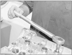
10.41b Torque-tightening the cylinder head bolts
