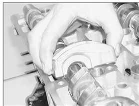
9.12b ... and remove the camshaft bearing caps
