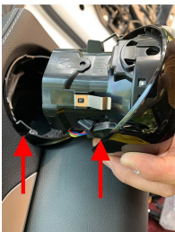
THE TOP LOGO IS FACING UPWARDS AND THE CORRESPONDING PIN IS PUSHED INTO THE AIR VENT
