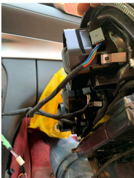
INSERT THE LAMP HOLDER OF CENTRAL CONTROL AIR OUTLET
