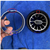
DISTINGUISH THE SIZE OF THE BUCKLE OF THE RED RING AND THE BASKET RING
