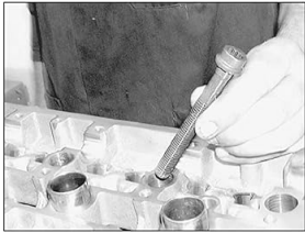
10.40 Inserting the cylinder head bolts
