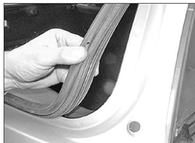
25.56 Peel back the glass hatch aperture seal
