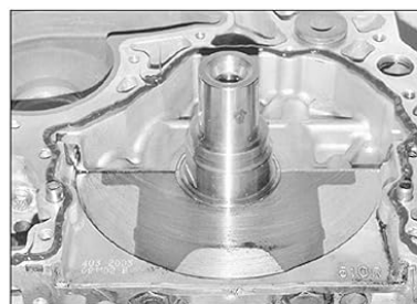
12.11 Apply a bead of sealant to the cylinder block mating surface
