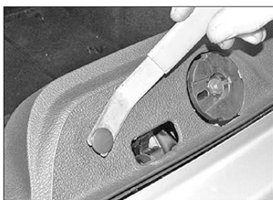
25.57 Unclip the trim upper securing clip
