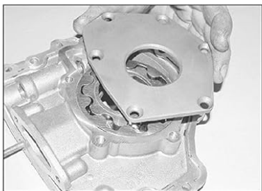
12.6 Undo the Torx bolts and remove the pump cover
