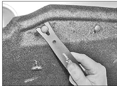
25.52 Release the securing clips . . .
