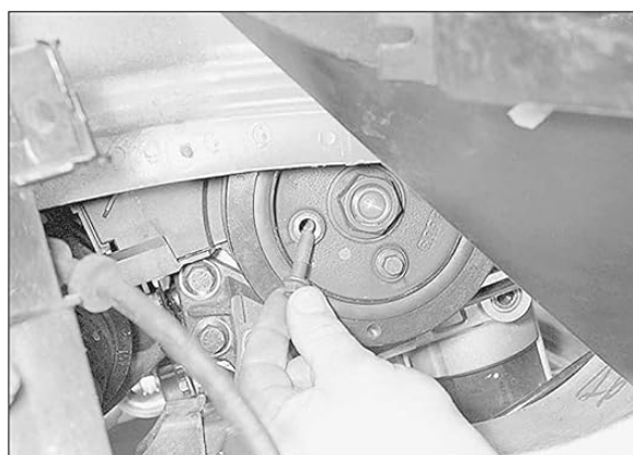
3.17a Loosen and remove two of the outer bolts . . .
