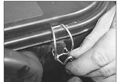
3.1b Work around the upper cover and prise open each of the tensioning clips
