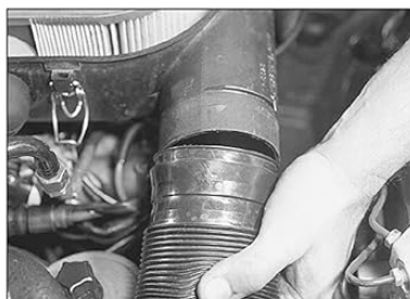
3.4b . . . and detach the inlet ducting from the air cleaner
