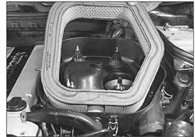
3.2c . . . and remove the air filter element
