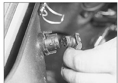
3.6 Unplug the wiring from the inlet air temperature sensor
