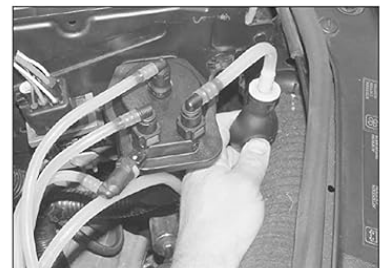
18.7 Squeeze the hand pump to fill filter with fuel
