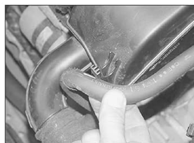
2.6 Disconnect the coolant hose from the air inlet elbow ...
