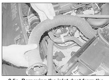
2.5c Removing the inlet duct from the front of the engine compartment – D7F engine
