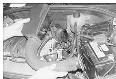
2.9c ... and remove the resonator box and duct from the air cleaner housing – K4J and K4M engines
