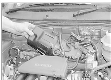
2.5b ... then lift the air cleaner from the engine – D7F engine
