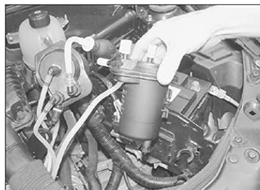
18.6 Dispose of the old filter and fit new filter into mounting bracket
