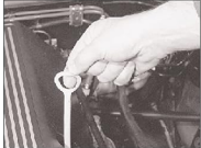
3.11a Removing the oil level dipstick . . .
