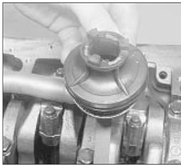
16.4b ... followed by the strainer from the oil pick-up tube (AAT engine)
