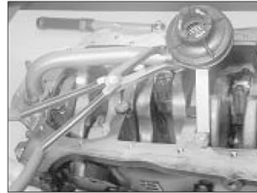
16.4a Using circlip pliers, remove the circlip ...
