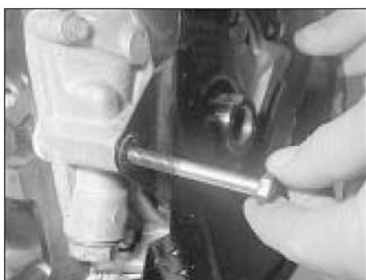
16.6a The inner timing cover is secured to the oil pump with the long bolts
