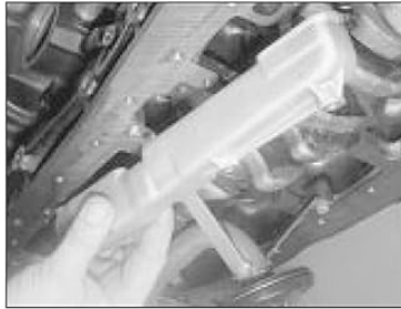
16.3b ... and remove the crankcase ventilation duct (AAT engine)
