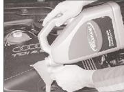
3.11c Use a funnel when adding oil to the engine
