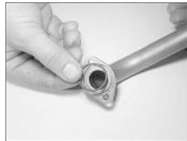
16.5d Removing the O-ring seal from the groove (AAT engine)
