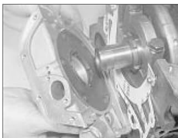
16.6b Remove the oil pump ...
