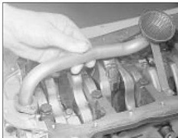
16.5c ... and remove the oil pickup tube (AAT engine)
