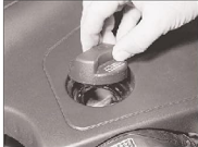
3.11b . . . and oil filler cap on the 2.5 litre 5-cylinder engine
