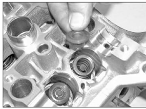
6.4a Remove the valve spring cap...
