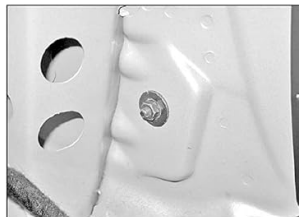
16.16 Undo the bumper retaining nut each side – Estate models
