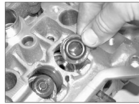
6.5 Lift off the spring seat
