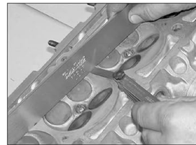
7.6 Use a straight-edge and feeler blade to check the cylinder head gasket face for distortion
